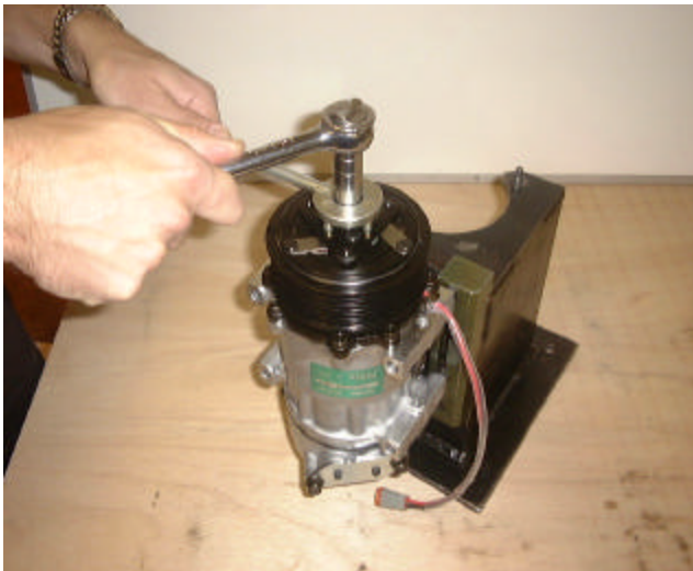
Fig.1 Removal of armature retaining nut
