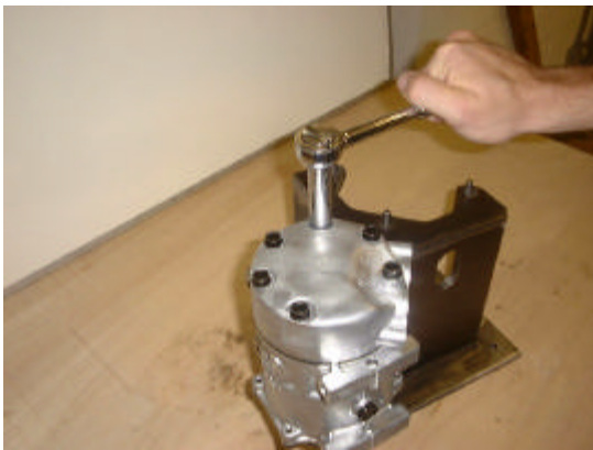
Fig.19 Removal of cylinder head bolts
