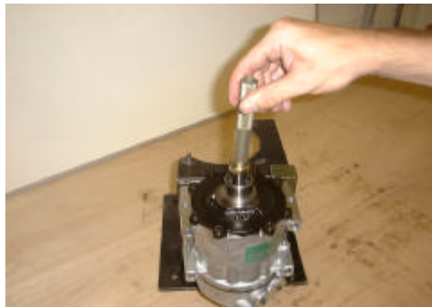
Fig.18 Replacement of lip seal
