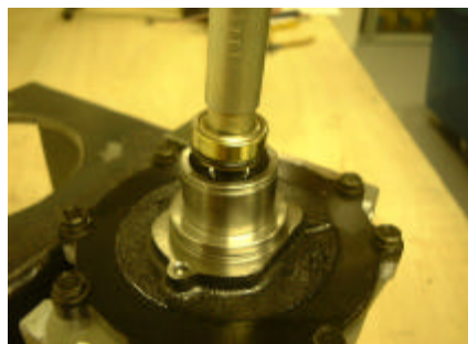
Fig.16 Shaft seal removal
