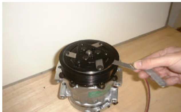
Fig.13 Check air gap with feeler gauges
